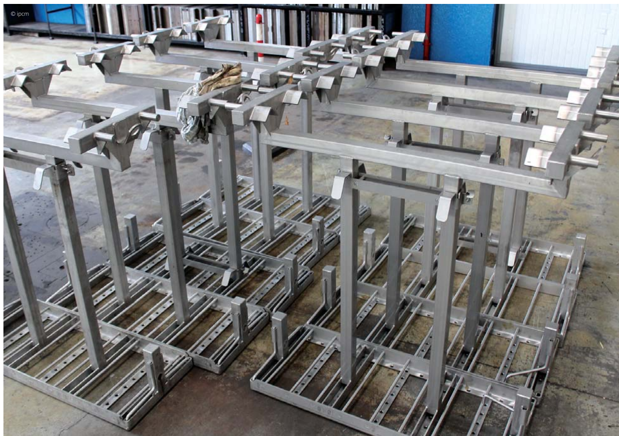
The frames for loading the two sides of the moulds to be cleaned.
