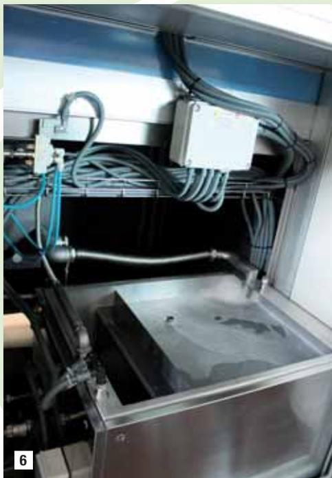
**6** The buffer tank with the water-based cleaning solution that helps the company to avoid production standstill during the maintenance operations.
