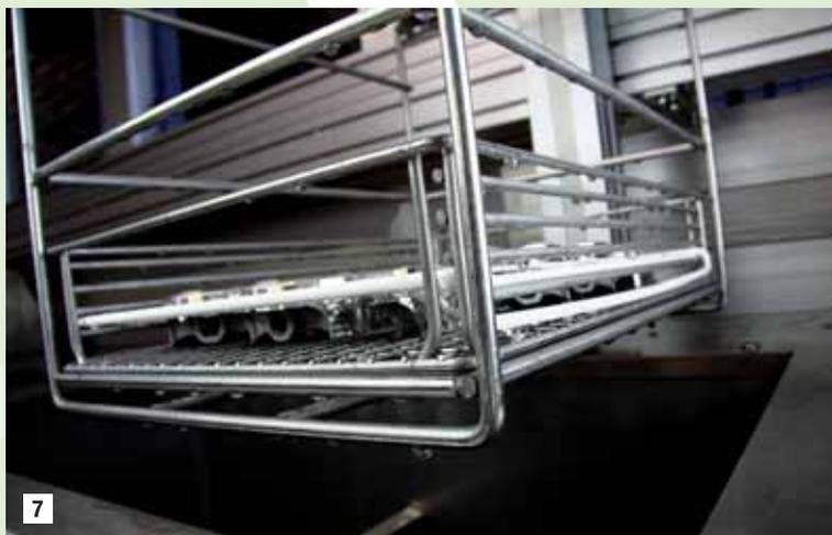
**7** Meteor Piston uses cleaning baskets with adjustable Teflon-coated racks to avoid any damage to the pieces.
