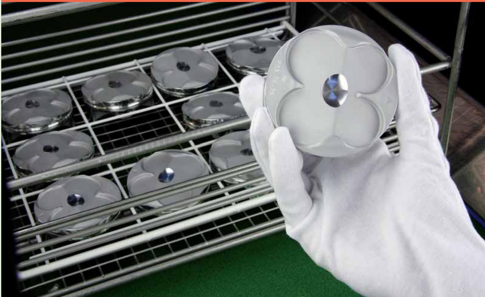
Opening picture: Pistons produced by Meteor Piston has extremely complex profiles and ovalities.
