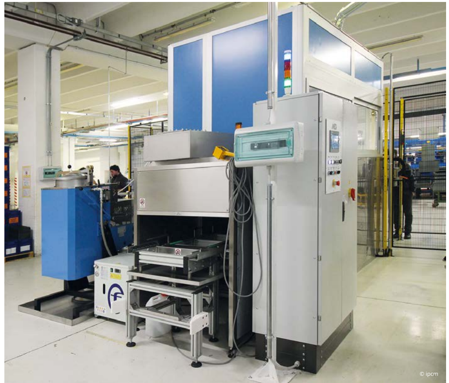
The additional oil separator for distilling HFE halogenated solvents and the unloading area.
