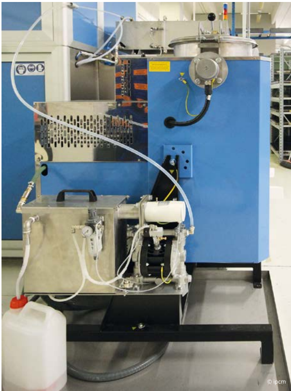
The additional oil separator for distilling HFE halogenated solvents and the unloading area.
