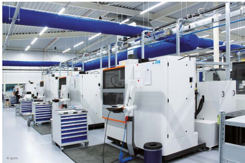
A partial view of JOB Precision's extensive equipment fleet (left) and some wire electrical discharge machining (WEDM) systems.
