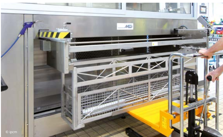
The entry area of the machine, customised to facilitate the loading of heavy components by a forklift.
