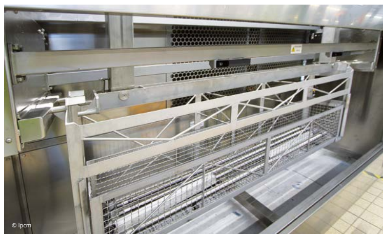
The entry area of the machine, customised to facilitate the loading of heavy components by a forklift.
