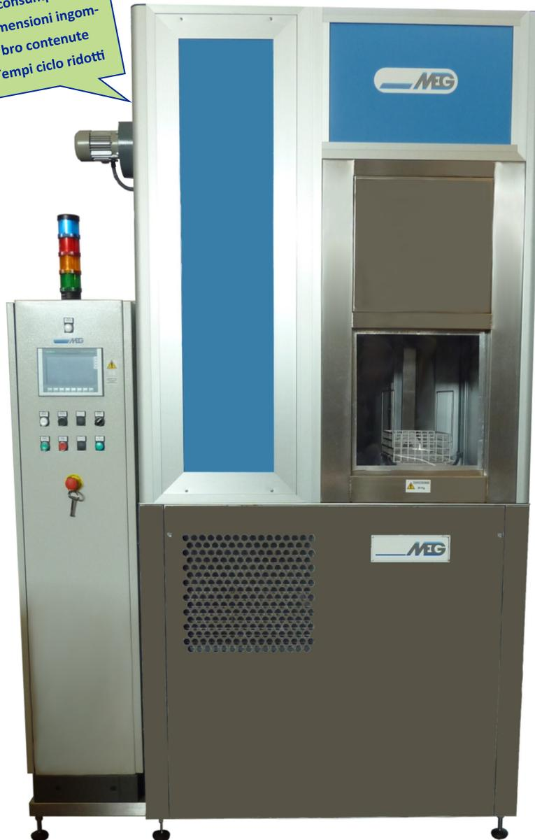
The **2S 24/12-P-F PCT+TA 20/1** is our standard version of automatic ultrasonic degreasing machine with Total Heat Pump and Boiling Tank. The machine was specially designed for use with new generation of environmentally-friendly fluorinated solvents, non-ozone depleting and low boiling, which contribute, together with the **Total Heat Pump**, to a considerable reduction in energy consumption.
