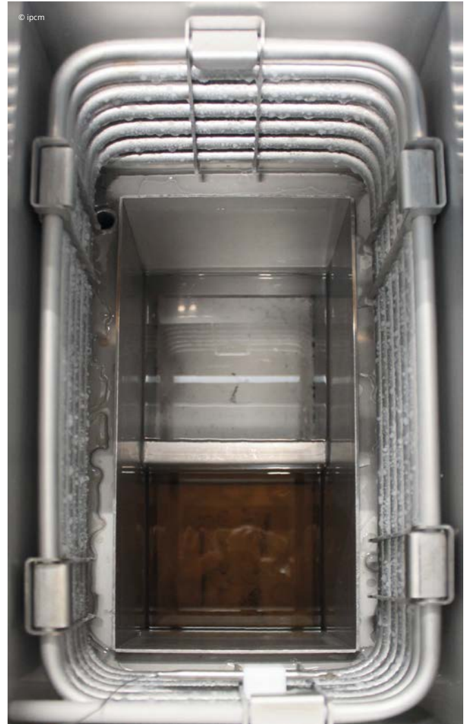
The inside of the multi-function cleaning chamber.
