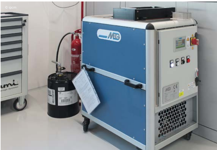
The first dental implant machining stage, with state-of-the-art sliding-head lathes and the HFE solvent system for the preliminary cleaning phase.
