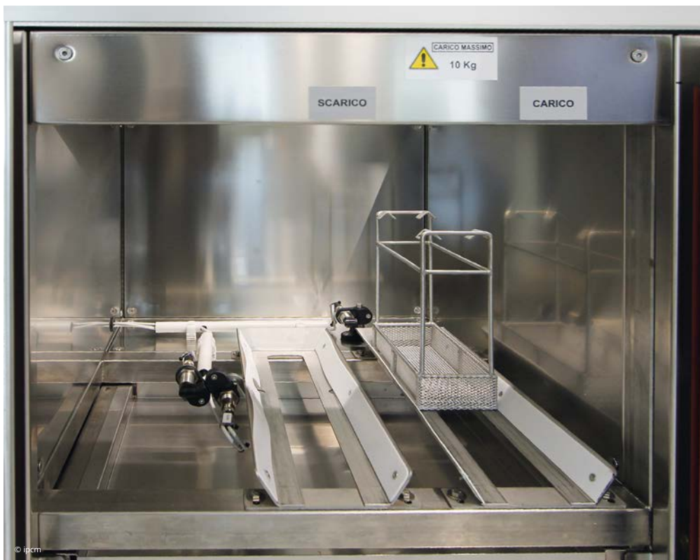
The loading/unloading station of the prosthetic component cleaning plant.
